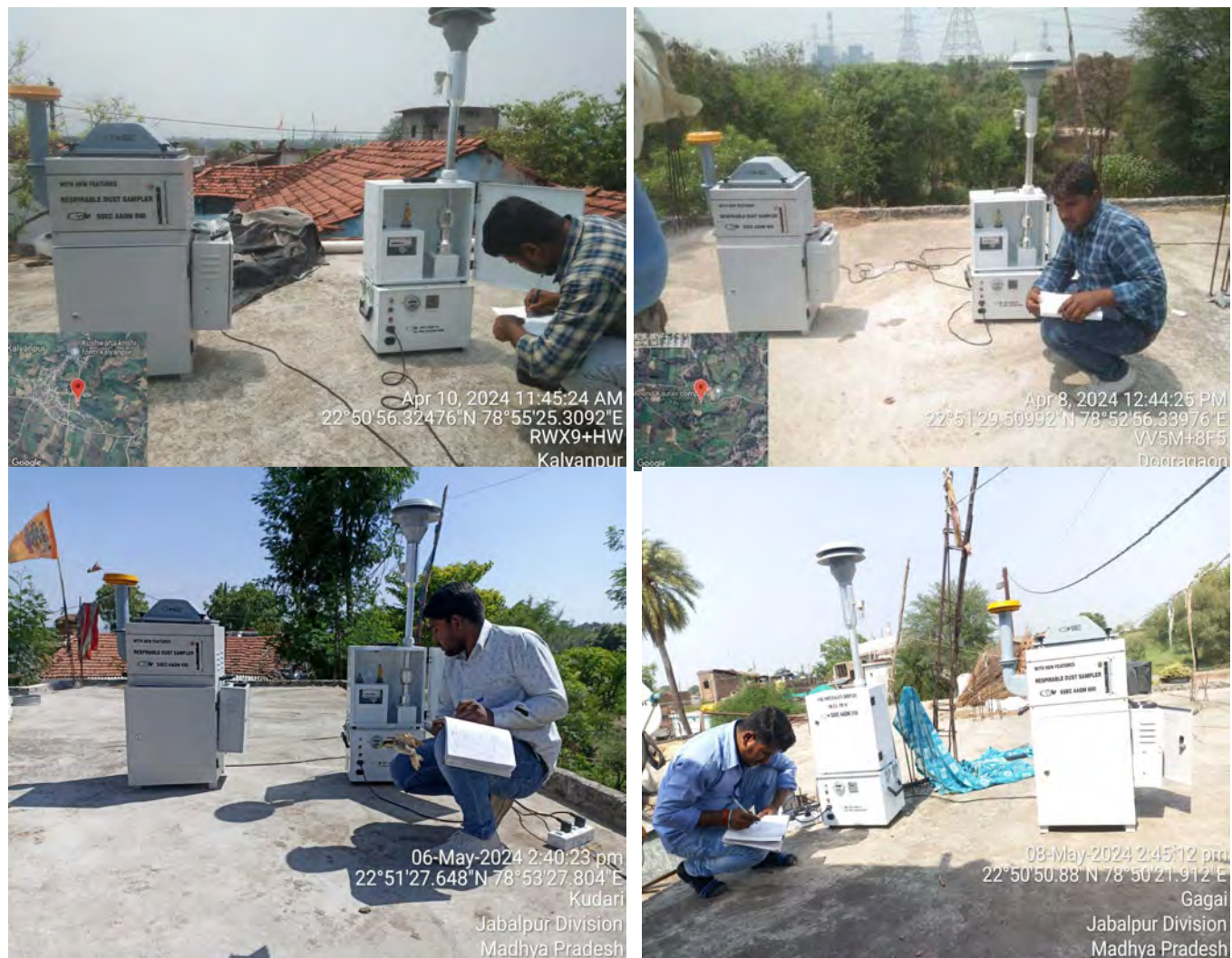
Figure 3-38: Ambient Air Quality Monitoring
