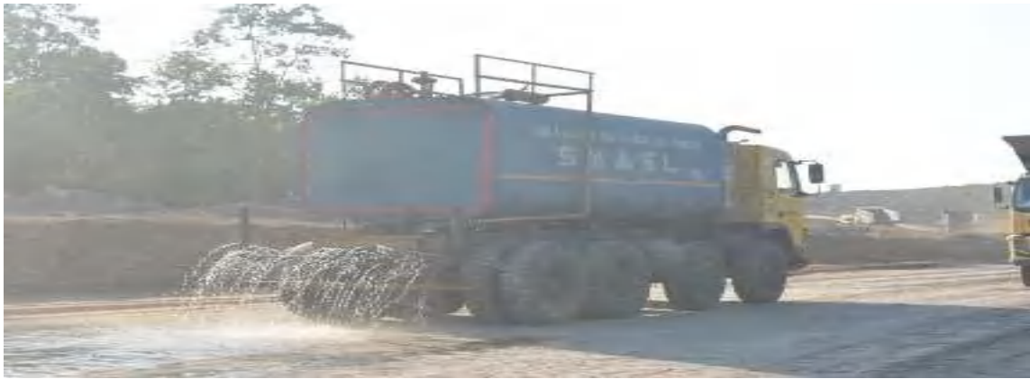
Water Sprinkling on Haul Roads inside Mines
