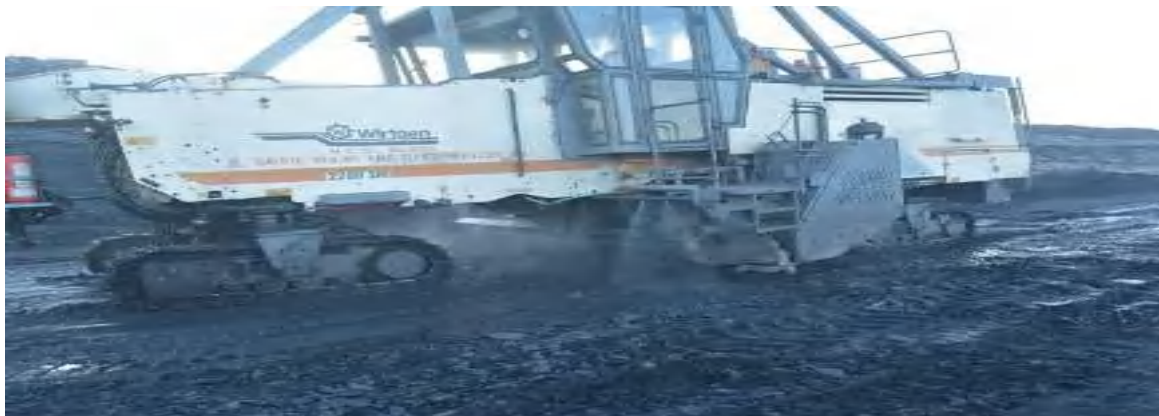
Interlocked Dust Suppression arrangement in Surface Miner
